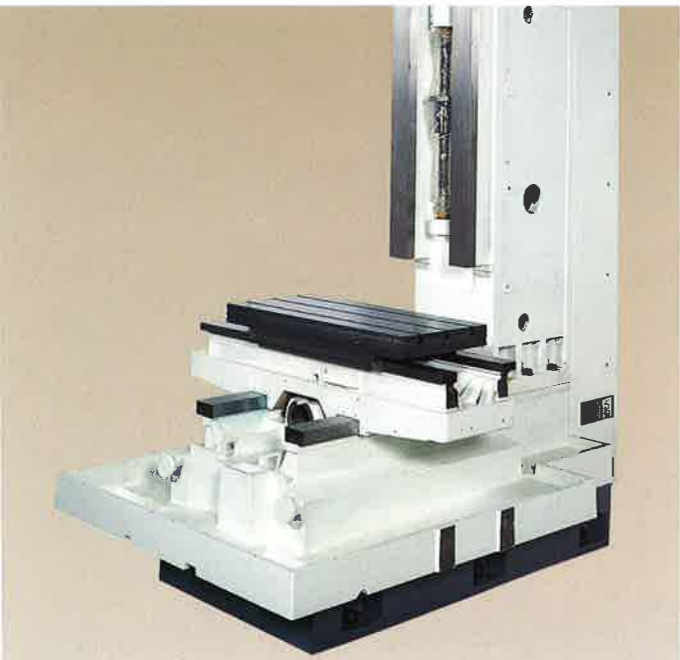
Precision Slide Way, ground after high-frequency hardening High-rigid basic construction
